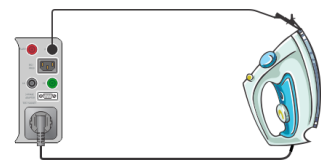
Substitute leakage test for Class I device
