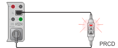
Active polarity test
