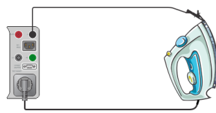
Earth bond test
